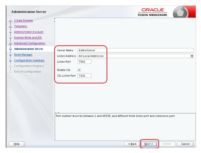
**Note**: The default Listen port is 7001 and SSL port is 7101. This could be changed to any other available port. Ensure to make a note, of this port since the same is required for launching the Admin console, post domain creation.
